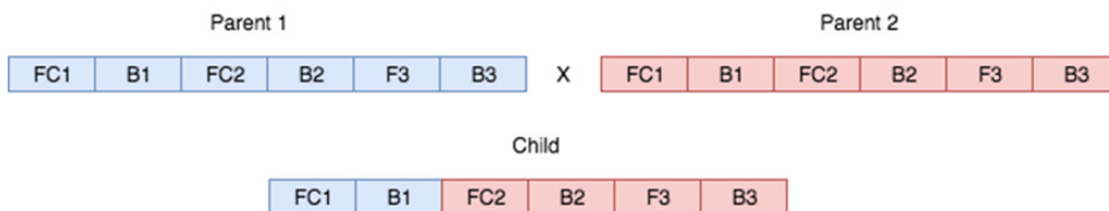
Figure 6.4: We will be passing the weights of each parent of each parent down to each child. Each child will receive a random amount of weights from each parent. In the above case, the child received the first two "genes" (FC1 and B1) from parent 1 and the remaining four from parent two, but this could be random permutation.
