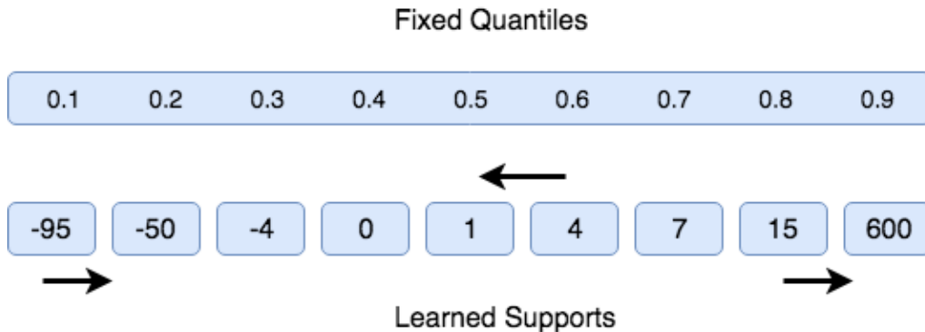
Figure 7.21 : In quantile regression, rather than learning what the probabilities are that are assigned to a fixed set of supports, we learn a set of supports that correspond to a fixed set of probabilities (quantiles). In this figure you can see the median value is 1 since it is at the 50 th percentile.
