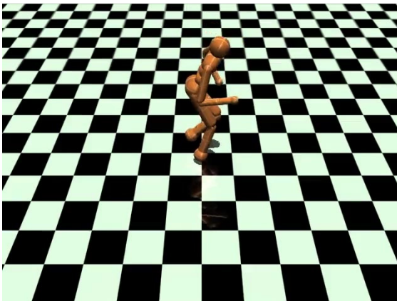
Figure 6.11: The 3D Humanoid environment provided by the gym library. This is high dimensional problem where the objective is for the humanoid to walk forward. With just one machine an ES was able to “solve” this problem in 11 hours, but by using 80 computers they were able to produce an agent in 10 minutes.
